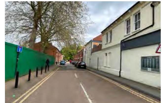
Figure 33: Bollards used to prevent vehicles from blocking the footway along Buckingham Street.
